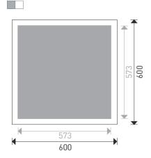
Fire reaction pre and postpainted tiles: A2s1do Release of dangerous sustances: none Flexion resistance: Classe 1 Durability galvanized tiles: B Durability pre and post-painted tiles: C
